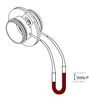
The Iris damper features two measuring ports. One is on each side of the apeture. A manometer connected across the ports will measure differential pressure (pressure drop). If you know the orifice configuration and the pressure drop, airflow (CFM) can be calculated.
